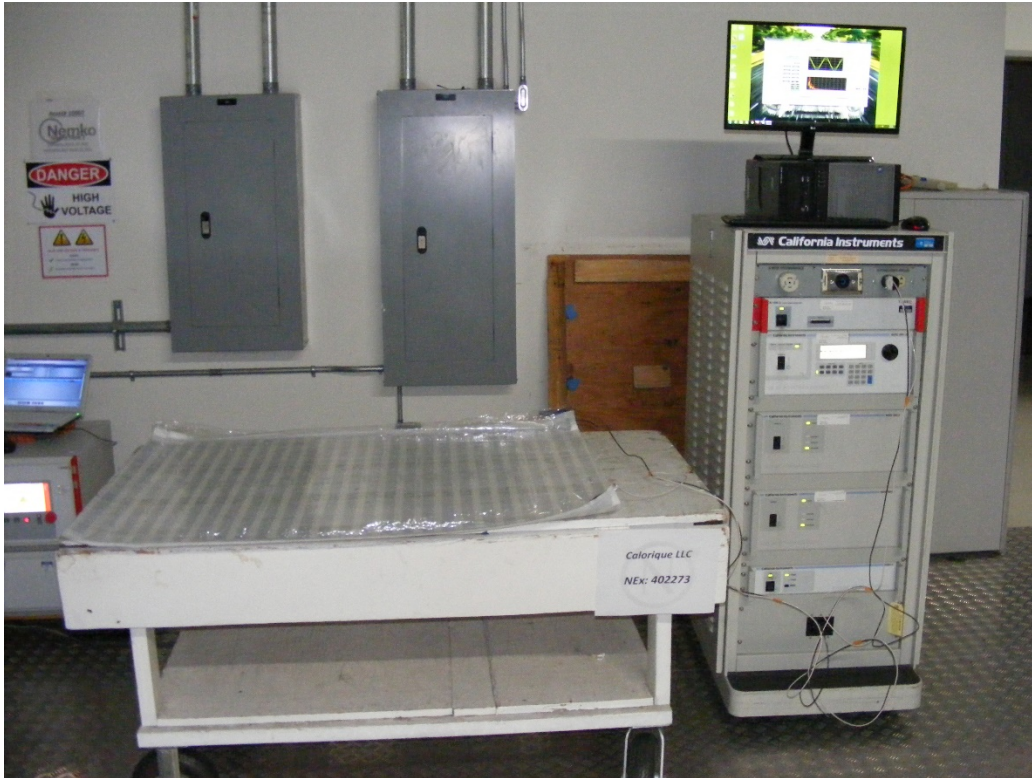
Figure 8.5-1: Voltage fluctuations and flicker setup photo
