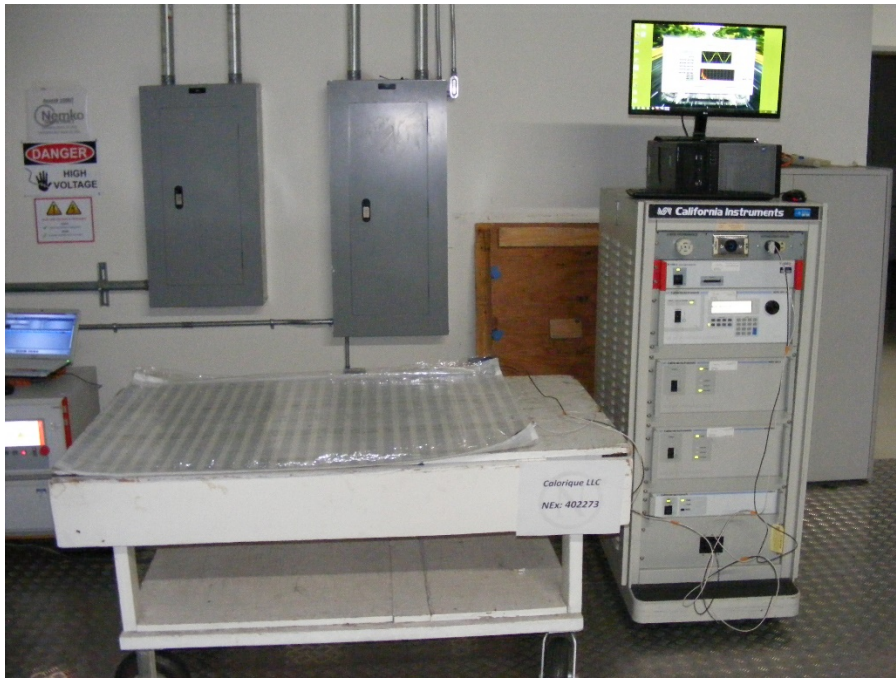
Figure 8.4-1: Harmonic current emissions setup photo
