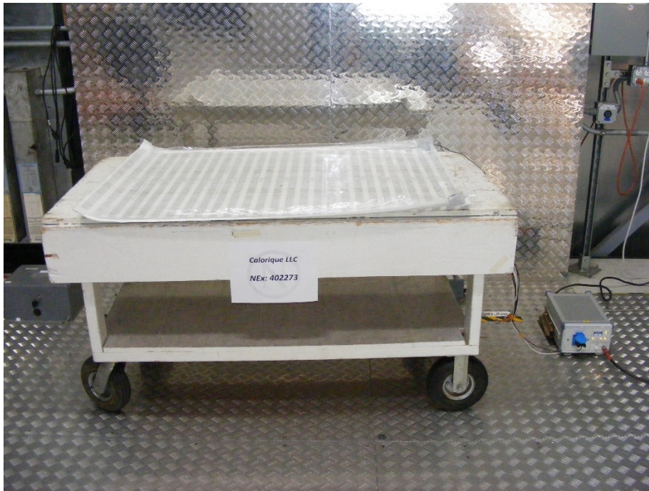
Figure 8.2-2: Conducted disturbance at mains port setup photo
